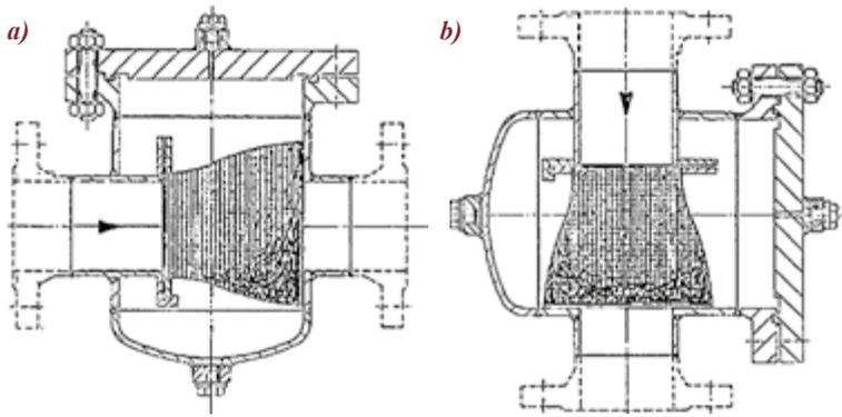
**Figure 5:** W-Filter (dirty) in horizontal flow path (a) and in vertical flow path (b)
