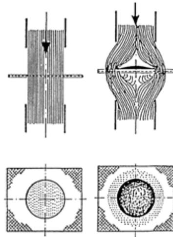
**Figure 3:** Flow path in a T-Filter under clean (left) and dirty conditions (right)
